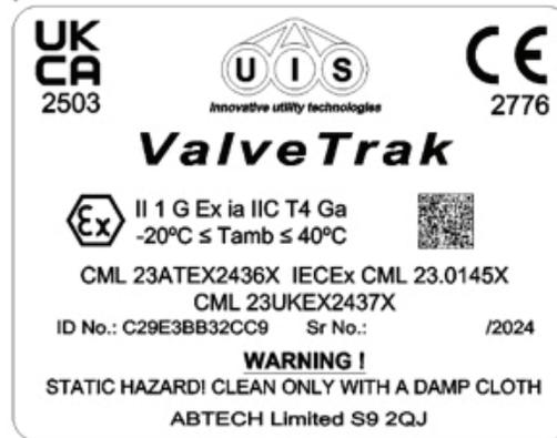
Valve Trak is a self-contained piezo sounder with integral Bluetooth transceiver. The equipment is powered from internal non-replaceable primary cells, and comprises; the cells, circuit board, and piezo sounder, mounted within a non-metallic enclosure. The equipment is intended for the location of gas service points and normally operates in low power standby mode and when pinged by a nearby Bluetooth transmitter, emits an audible tone to allow the equipment to be located.
