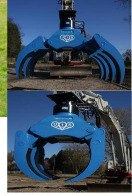
Before using the UIS Power Handler<sup>™</sup> you must always ensure that the carrier excavator is capable of lifting the PH along with a full capacity load. Failure to do this may result in serious injury or even worse.
